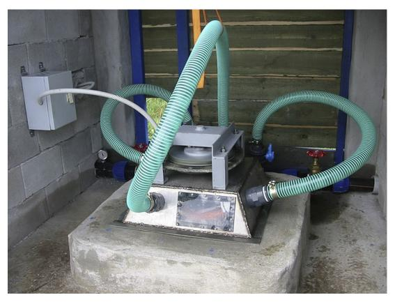
Fig. 4. A 500 W locally manufactured pico-hydroelectric plant.
